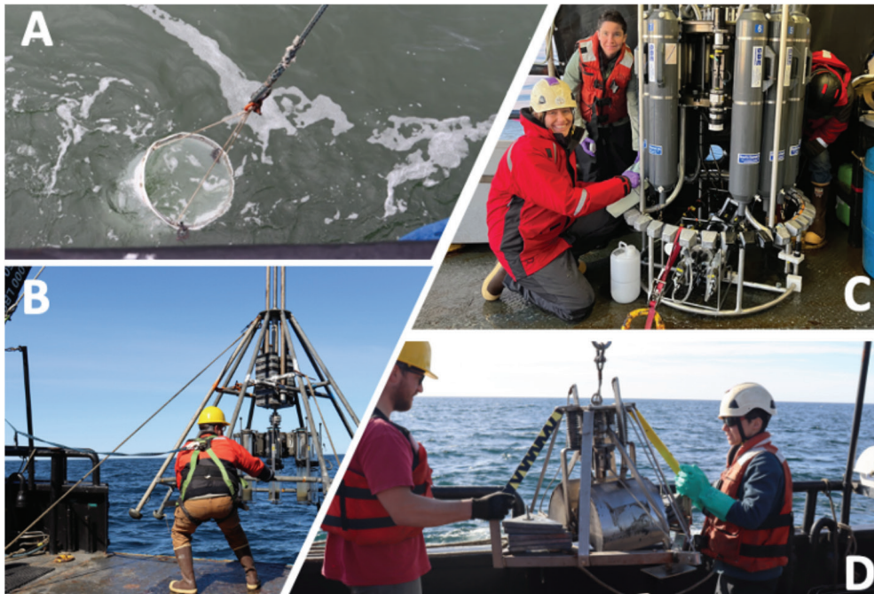
FIGURE 17. Sampling operations aboard the R/V Norseman II . A) net tow B) MC-800 multi-core C) CTD Rosette D) Smith-McIntyre grab.
